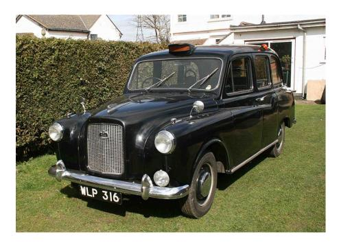
42. In 1962 Winchester Automobiles (West End) Ltd introduced its Series I cab, which was the first to have a glass reinforced plastic ("GRP") body. This was followed by the Series II in 1965, the Series III in 1966 and the Series IV in about 1967. None of these models was successful and few were made. The last Series IV was made in February 1971 and sold later that year. The Winchester is shown below:
