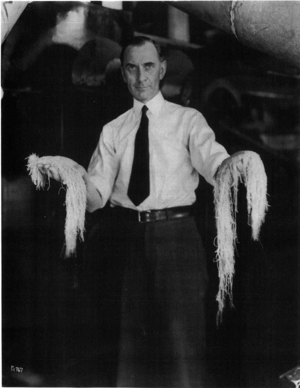
#4 - A Photograph showing the shreds which have been removed from the Carrier Belt.
